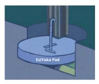
3. Lower pad into excavation and adjust as required. Pad maybe removed if required.
