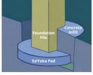
4. Place foundation pile in position. Piles may be cut to length and braced using bearer or hand while concrete infill is poured.
