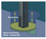
2. A plywood compactor can be cut and fixed to a suitable length of timber for the purpose of compacting a granular fill layer such as sand.
