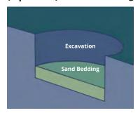
1. Spade in required damp sand or granular fill and spread over bottom of excavation.
