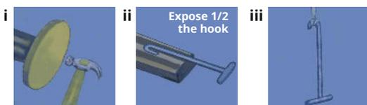
i. Fix a ply compactor with nails to a suitable length of timber. ii. Fix supplied hooks to a suitable handle as shown. iii. Or tie the hook to a rope.
